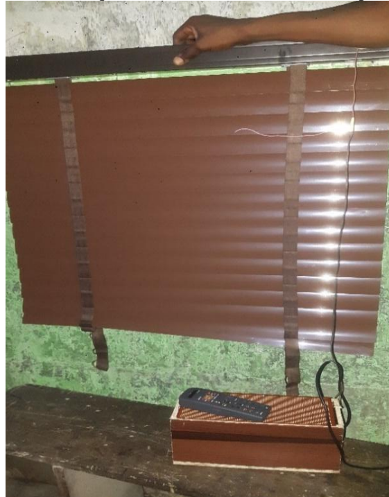
Figure.10. Constructed window blind in close operation.
