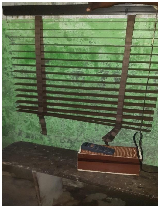
Figure.11. Constructed window blind in open operation.
