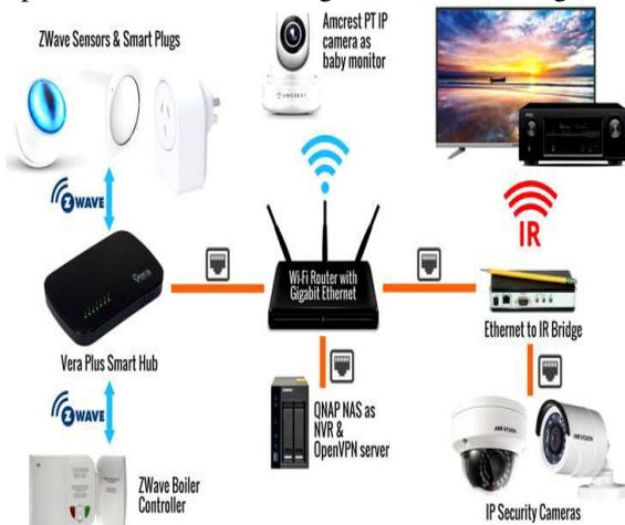
Figure. 6. The Z-Wave Network
