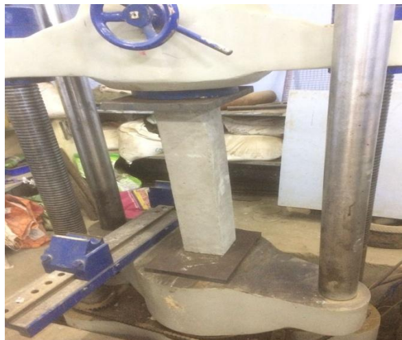
Figure. 3. Testing Of Conventional Column
