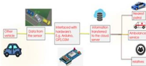
Figure.4. System Architecture
