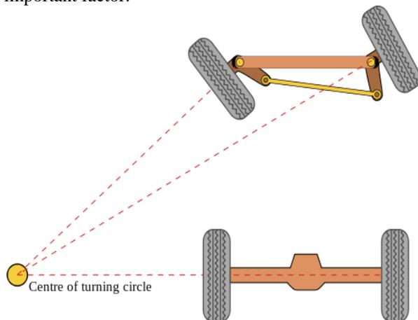
Ackermann steering geometry is a geometric arrangement of linkages in the steering of a car or other vehicle designed to solve the problem of wheels on the inside and outside of a turn needing to trace out circles of different radii. The intention of
