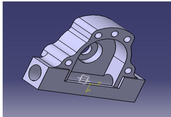
Figure.4. Steering Casing
