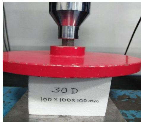
**Figure.4. Testing of 100mm X 100mm X 100mm having density 30 Kg/m<sup>3</sup>**
