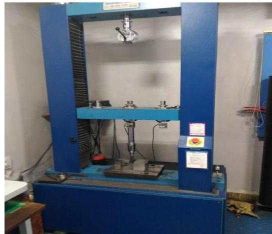
**Figure.3. Universal testing machine of capacity 9800N**
