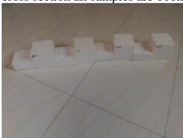
**Figure.2. 8 Sample of size 100mm X 100mm X 50mm and 100mm X 100mm X 100mm having density 22kg/ m<sup>3</sup> and 30Kg/ m<sup>3</sup>.**
