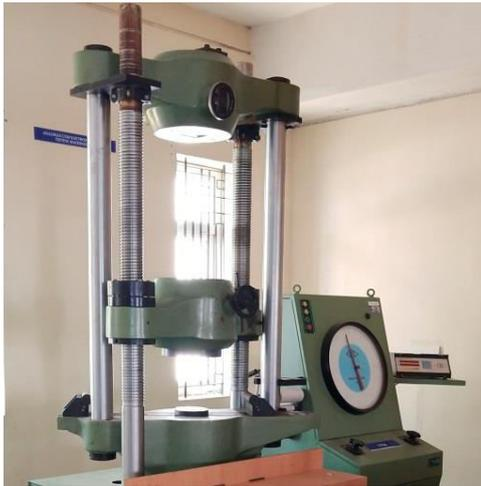
Fig.4.1. Universal Testing Machine
