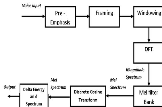
**Figure.3. MFCC Block Diagram [8, 9]**
