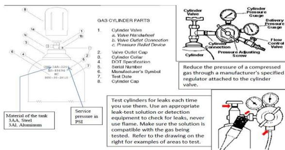
Figure 7.1 compressed gas cylinder parts
