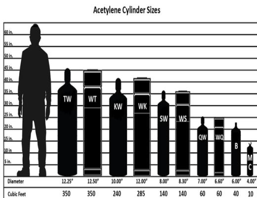
Figure 1.3 Acetylene Cylinders
