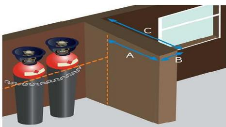
Figure.4.1. Use of a partition to achieve the minimum recommended separation distances
