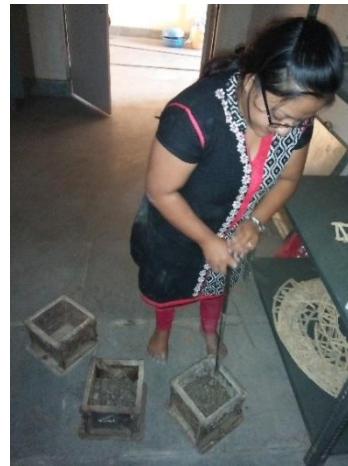
Figure. 6. Making concrete cubes
