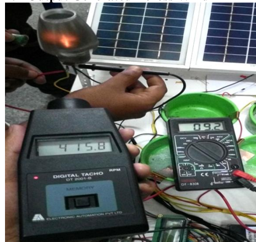
Figure.2. Output Voltage and Speed Across Wind Turbine
