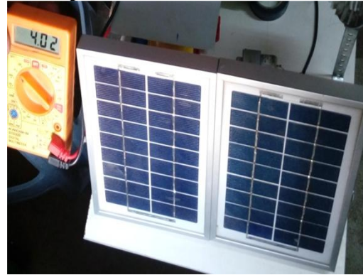
Figure .1 .Output Voltage of Photovoltaic Panel
