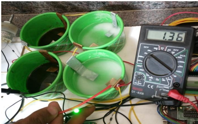
Figure.5. Output Voltage across Saline Water and Garbage Waste
