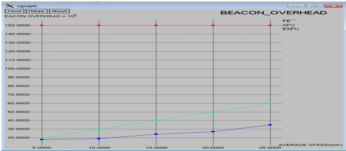
Figure.7. Beacon Overhead Vs Speed(m/s)
