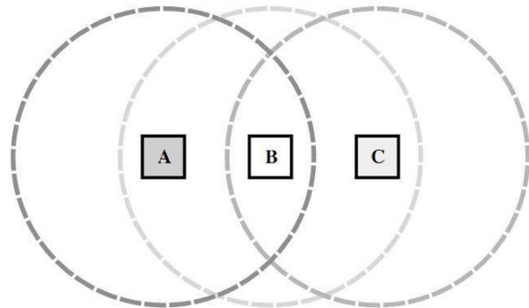
**Figure.1. A Mobil Ad hoc network of three nodes, where nodes A and C must discover the route through B in order to communicate.**
