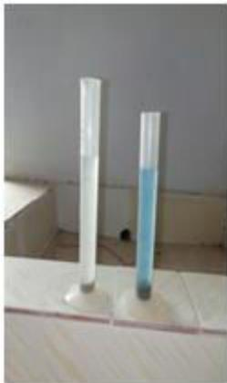
The free swell index of clay for untreated soil is found to be 50%. So degree of expansion is very high.
