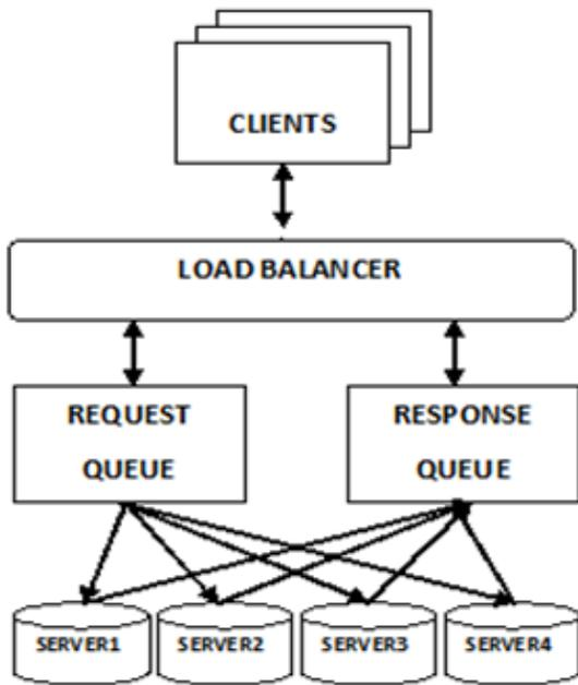
Fig 2 Flow of Load Balancing.
