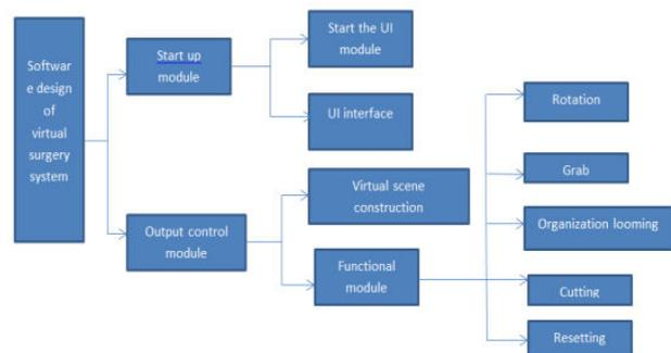
**Figure.1. Software system structure diagram**
