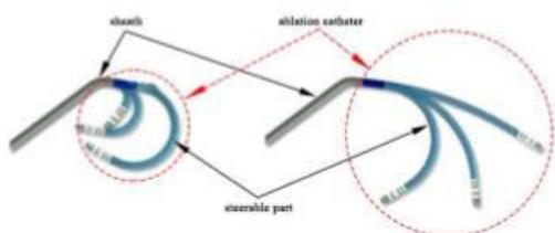
**Figure.4. the interaction between the sheath and the steerable catheter.**
