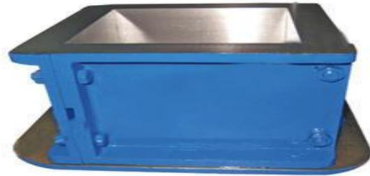
Figure.2. (Cube Mould)
