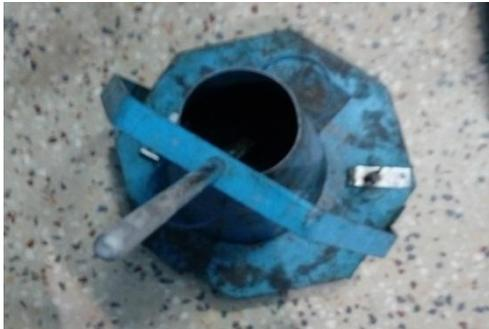
Figure.1. (Slump cone)
