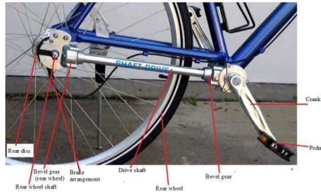
**Figure.2. Component of cycle**
