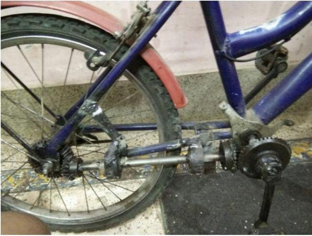
**Figure.4. Fabricated setup of modified gear and shaft transmission system**
