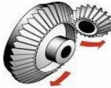
**Figure.3. Bevel Gear**
