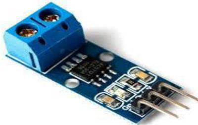
Figure.3. Current sensor module
