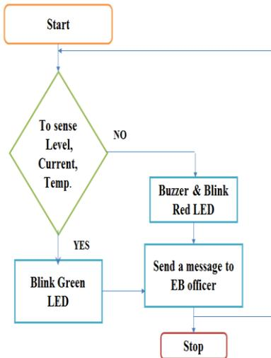
**Figure.5. Flow chart for Software implementation**
