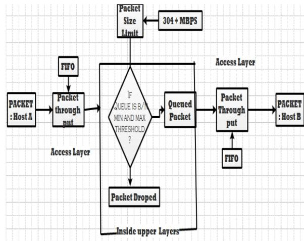
**Figure.4. Modeling WRED Algorithm congestion detection**
