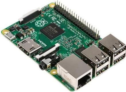
**Figure.2. Raspberry Pi Model B**
