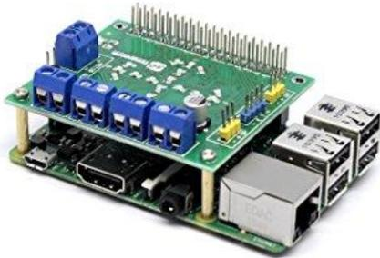
**Figure.3. Stepper motor hat for Raspberry Pi**
