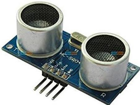
**Figure.4. HC-SR04 Ultrasonic sensor**
