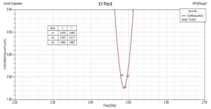
**Figure.4. VSWR Plot of 1/6 th patch of hexagonal antenna**
