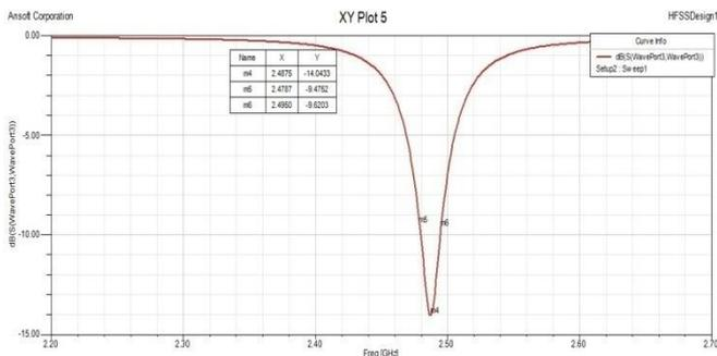
**Figure.3. Return loss of 1/6 th patch of hexagonal antenna**
