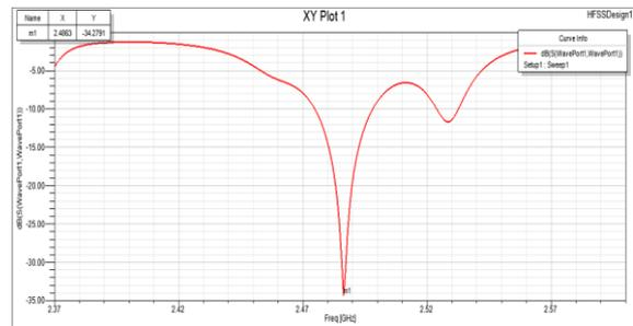
**Figure.11. Return loss of 4 x 1 Microstrip Patch Antenna array with EBG**
