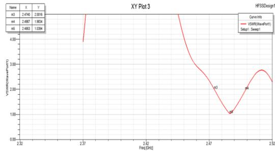
**Figure.12.VSWR of 4 x 1 Microstrip Patch Antenna array with EBG**
