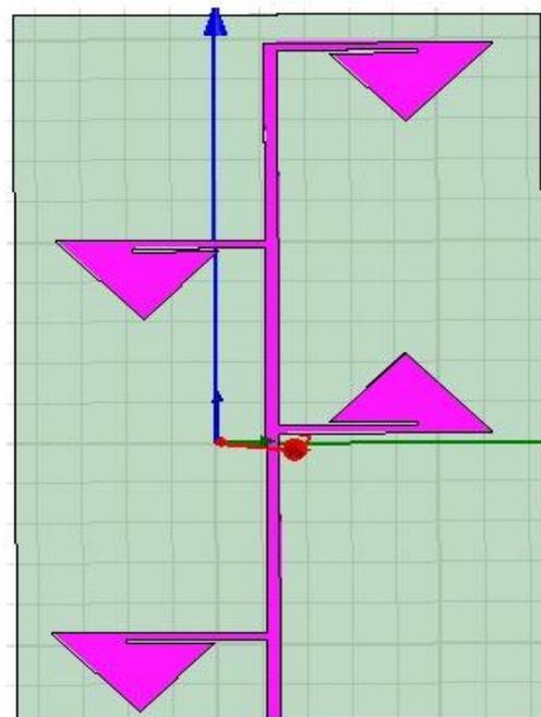
**Figure.6. 1/6 4X1 patch array without EBG**
