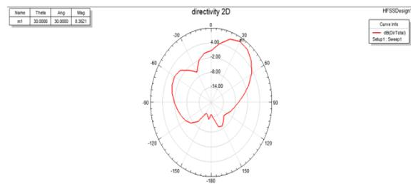
**Figure.13. Radiation pattern of 4 x 1 Microstrip Patch Antenna array with EBG**
