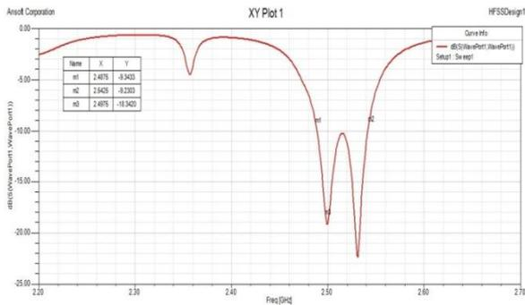
**Figure.7. Return loss of 1/6 4X1 patch array without EBG**
