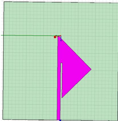
**Figure. 2. 1/6 th patch of hexagonal antenna**
