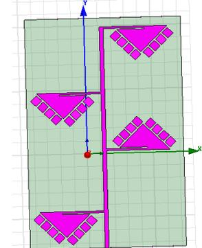
**Figure.10. 1/6 4X1 patch array antenna array with EBG**
