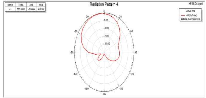
**Figure.5. Directivity of 1/6 th patch of hexagonal antenna**
