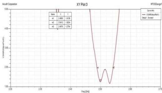
**Figure.8. VSWR of 1/6 4X1 patch array without EBG**
