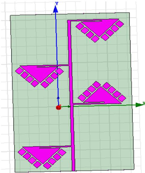
**Figure.1. Evolution of simple patch Configuration of (a) 1/6 th patch of hexagonal antenna, (b) 4X1 path array without EBG, (c) 4X1 path array with EBG**
