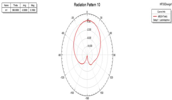
**Figure.9. Radiation pattern of 1/6 4X1 patch array without EBG**
