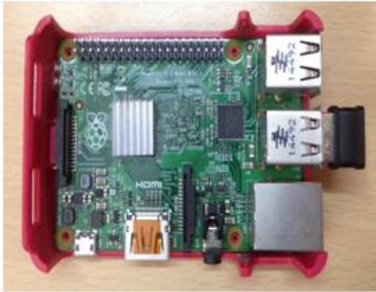
Figure. 3.2 Raspberry Pi 2 Module
