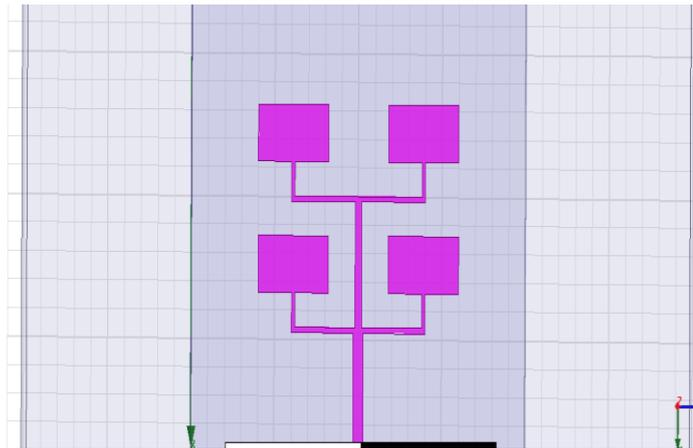
Figure .4. Four element Planer array HFSS model
