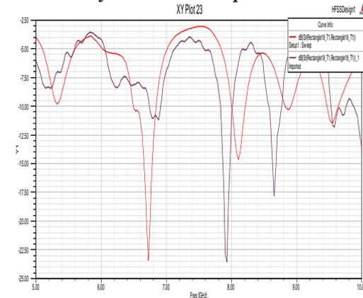
**Figure.13. comparison plot between fabrication and simulation**
