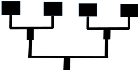
Figure.1. Four element corporate feed microstrip antenna array
