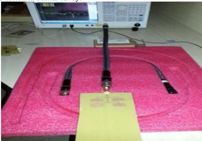
**Figure.11: Experimental setup for the measurement of planar array**
