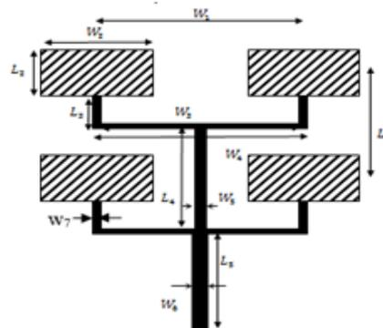
Figure.3. Proposed 2x2 corporate feed microstrip patch antenna
