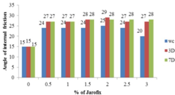
**Figure.7 Angle of internal friction v/s % of Jarofix content**
