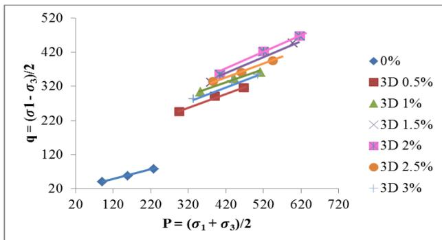
**Figure.4. Modified failure envelope (3 days curing)**
