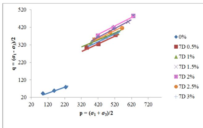
**Figure.5. Modified failure envelope (7 days curing)**
