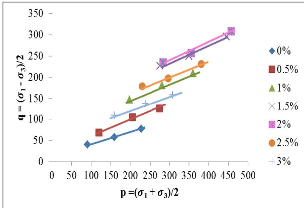
**Figure.3. Modified failure envelope (without curing)**
