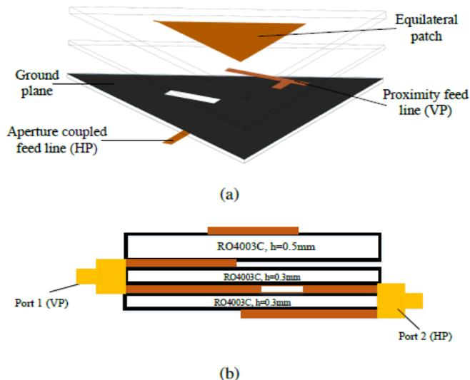
**Figure.9.** The (a) exploded and (b) side view of the dual-LP equilateral patch antenna. Both feed lines share a same ground plane [34].
