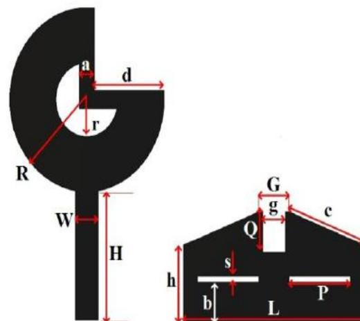
Figure. 3. Geometry of proposed RSMA [26].
