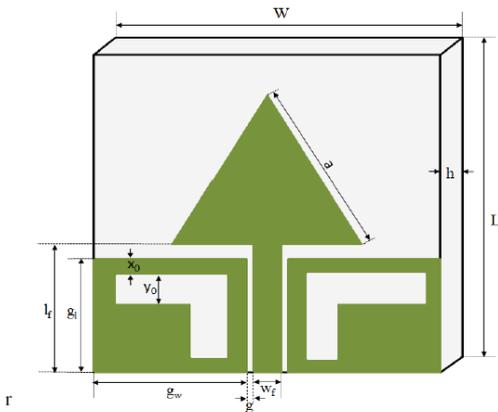
**Figure.4. Geometry of equilateral triangular patch[42].**
