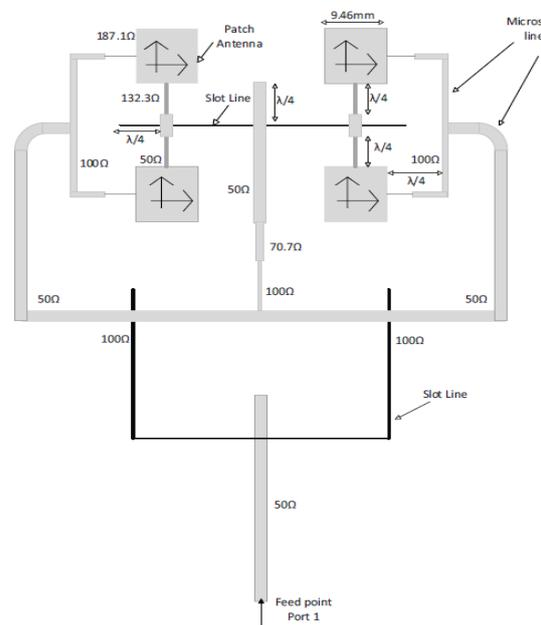
**Figure.10. (a) Geometry of array antennas with feed.**
