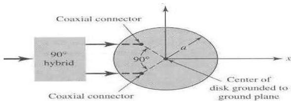
Figure.1. (c) Circular patch with coax feed [2].
