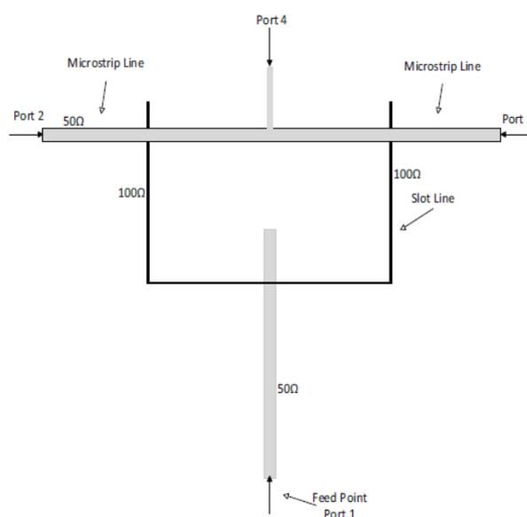
**Figure.10. (b) Basic configuration of triple feed structure.**
