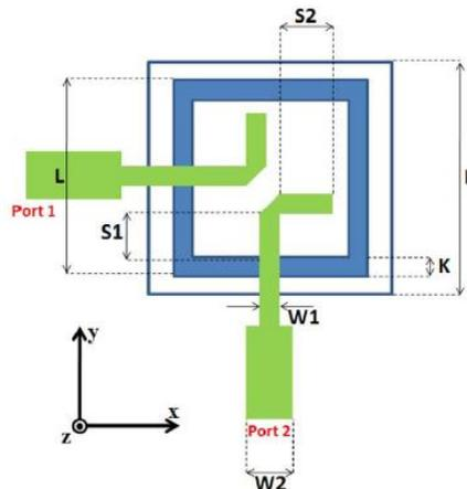
**Figure. 8. Geometry of square patch with dual feed [33].**
