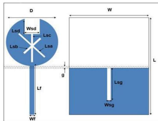
Figure. 2. Circular monopole antenna [23].
