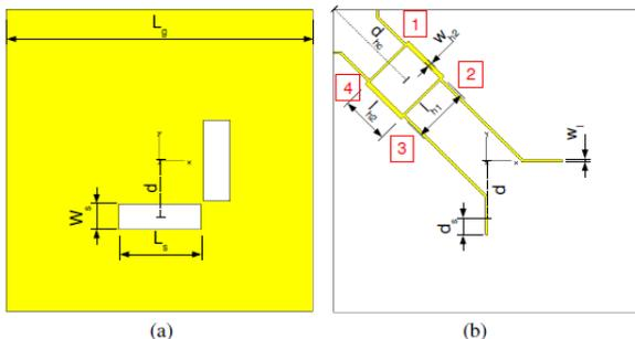
**Figure.6. (a) Ground plane: (a) front view of the upper layer (ground + slots),(b) back view (horizontally flipped) of the down layer (feeding lines) [31].**
