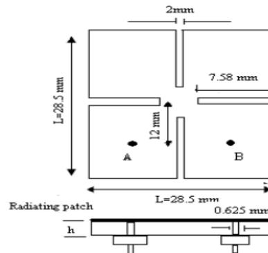
**Figure.7. Geometry of proposed square-fed flower-shaped Microstrip patch antenna [32].**
