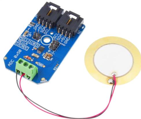
Figure.5. Shock sensor
