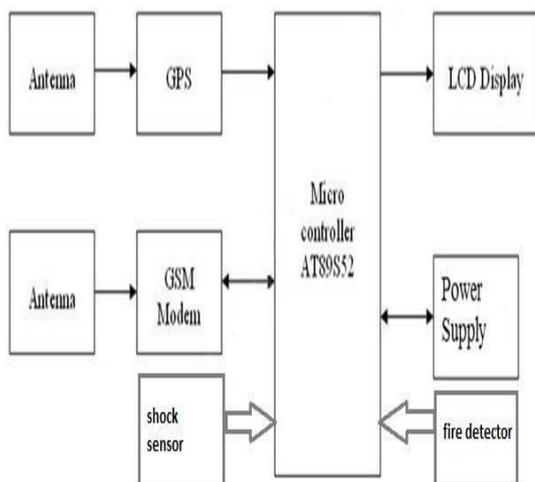
figure.1. block diagram of alert system
