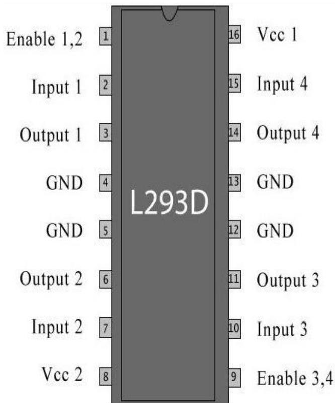
**Figure.3. Pin Diagram of L293D Motor Driver IC controller**
