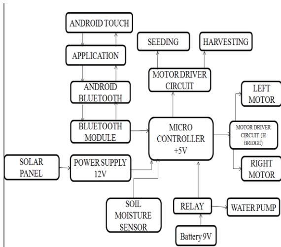
**Figure.1. Block diagram of Multipurpose Agricultural robot**
