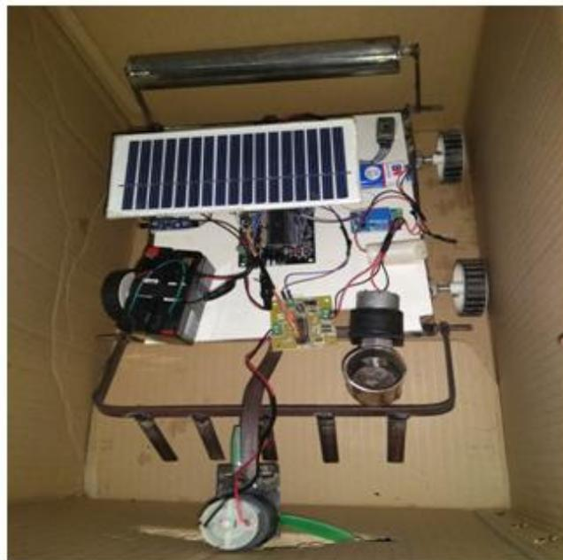
**Figure.2. Top view of Prototype models for plowing, leveling, seeding and water spraying operations**
