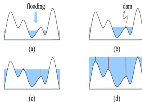
Figure.2. Watershed Segmentation Algorithm
