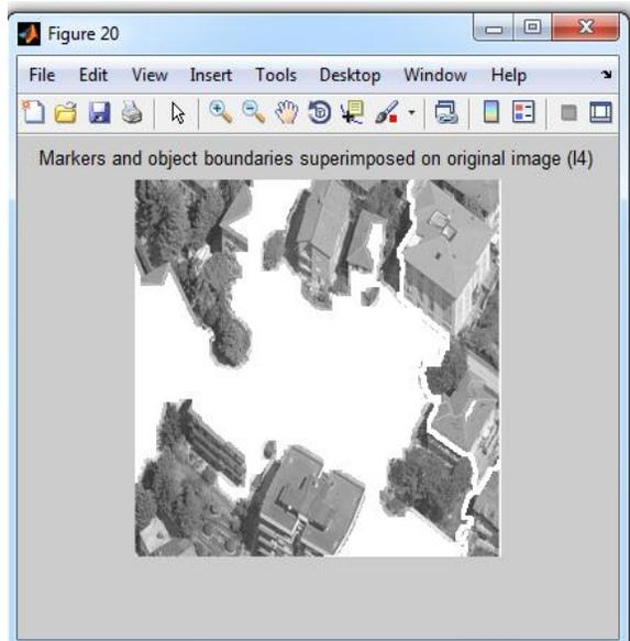
Figure.10. Super imposed image of marker and object boundaries.
