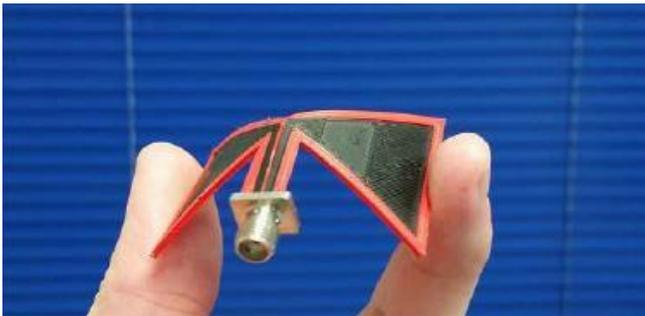
Figure .6. Bow-tie antenna after fabrication [8].
