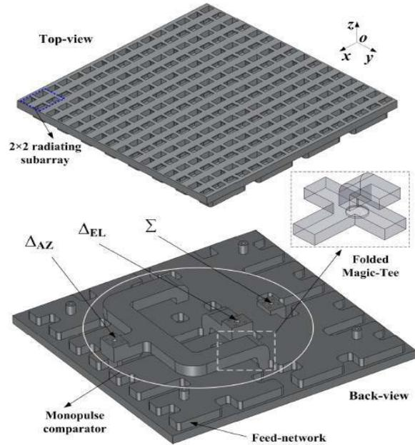
Figure.8. Configuration of the monopulse array [10]
