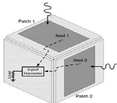
Figure.3.3-D cube for RF energy harvesting electronics.
