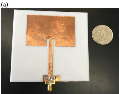
**Figure.11.** (a) Configuration of the microstrip patch antenna; (b) MPA after fabrication [13].
