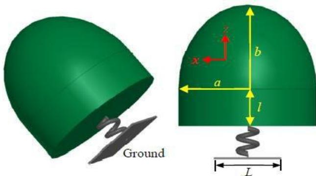
Figure. 7. Helical antenna design integrated with lens [9].
