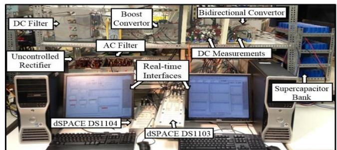
Figure. 2: General view of the dc microgrid and its control desk.
