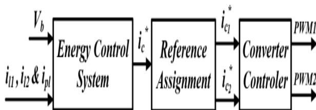
**Figure.3: Block diagram of the DC microgrid three layer control system.**
