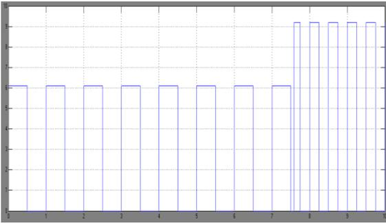
Experimental test results of CACC method and ACVC technique when pulse load frequency changes from 0.1-Hz to 0.2-Hz and its duty ratio increased from 20% to 40%.
