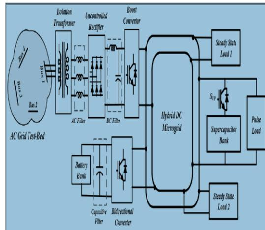
Figure.1. Schematic diagram of the hybrid dc microgrid under study.
