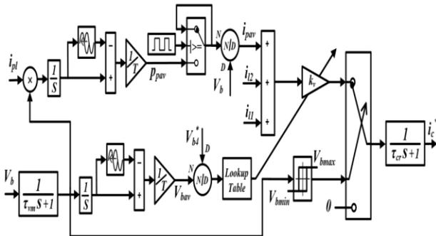
**Figure.9. Current-voltage control**
