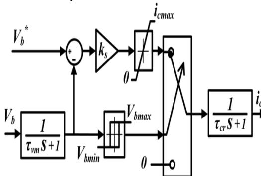
**Figure.6: Block diagram of the limit-base voltage control.**
