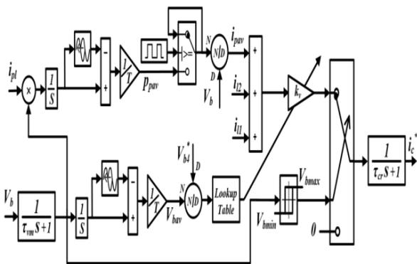
**Figure.8. Block diagram of adaptive current-voltage control.**
