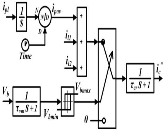
**Figure.7. Block diagram of continues average current control.**
