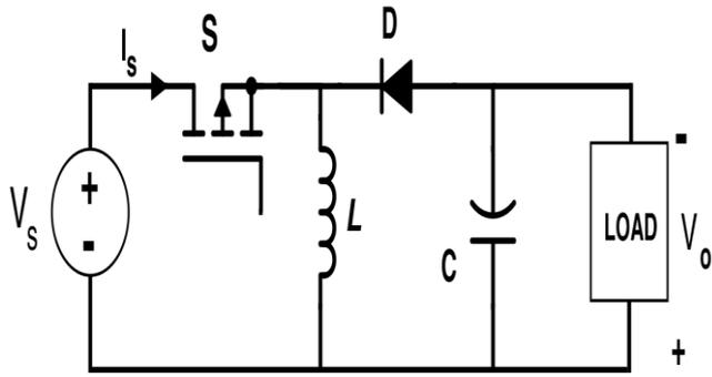
Fig 10: Buck-Boost Converter Circuit Diagram
