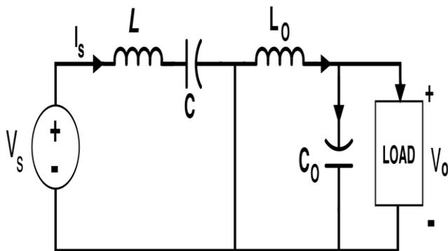
Fig 16: CUK Converter Circuit when Switch S is Off (Mode-II)
