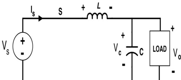
Fig 3: Buck Converter Circuit when Switch S is On (Mode-I)
