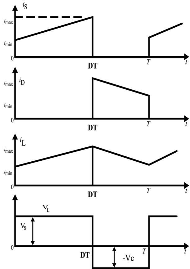
Fig 13: Supply Current, Diode Current, Inductor Current and Inductor Voltage respectively (Buck-Boost Converter) **CUK Converter:**
