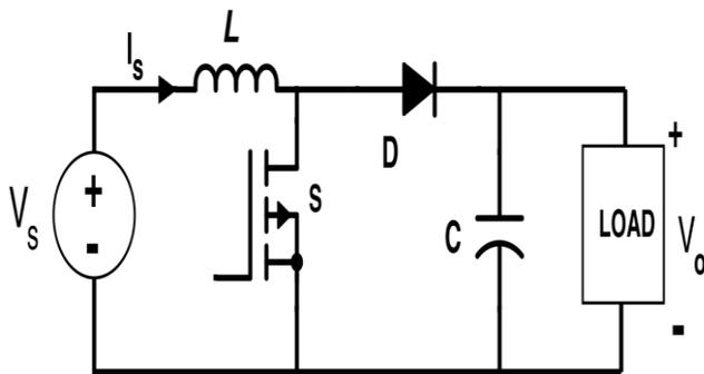
Fig 6: Boost Converter Circuit Diagram
