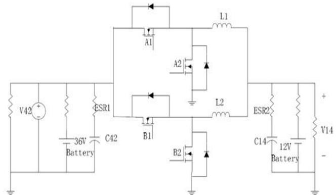
Fig1: Bidirectional DC/ DC Converter block diagram
