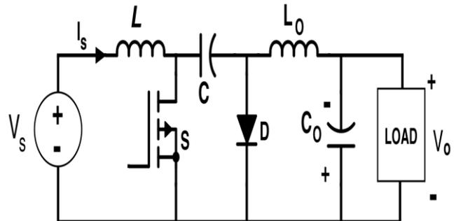
Fig 14: CUK Converter Circuit Diagram
