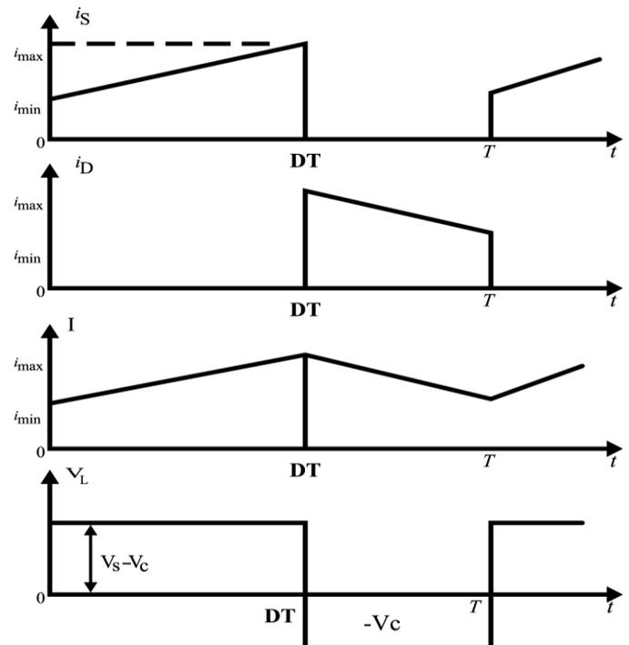
Fig 5: Waveforms of Supply Current  $I_s$ , Diode Current  $I_D$ , Inductor Current  $I$ , and Inductor Voltage  $V_L$ .
