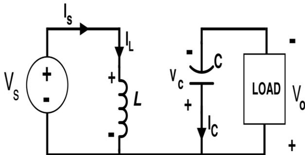
Fig 11: Buck-Boost Converter Circuit when Switch S is On (Mode-I)
