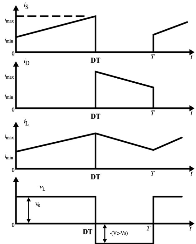
Fig 9: Waveforms of Supply Current  $i_s$ , Diode Current  $i_D$ , Inductor Current  $i_L$ , and Inductor Voltage  $v_L$ . (Buck Converter)
