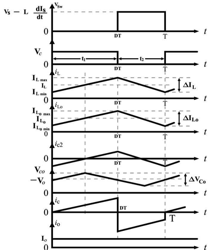
Fig 17: Switch (S) Voltage, Capacitor (C) Voltage, Inductor (L) Current, Inductor (L<sub>o</sub>) Current, Capacitor (C<sub>o</sub>) Voltage, Capacitor (C) Current and Load Current respectively for the Cuk Converter
