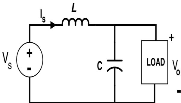
Fig 8: Boost Converter Circuit when Switch S is Off (Mode-II)
