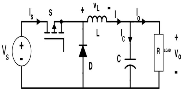
Fig 2: Buck Converter
