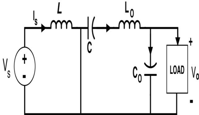
Fig 15: CUK Converter Circuit when Switch S is On (Mode-I)
