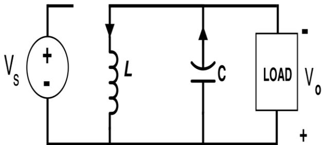
Fig 12: Boost Converter Circuit when Switch S is Off (Mode-II)
