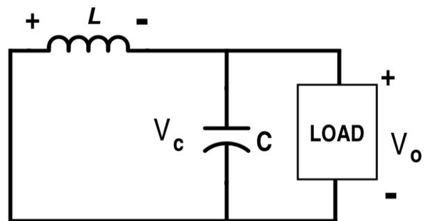
Fig 4: Buck Converter Circuit when Switch S is Off (Mode-II)
