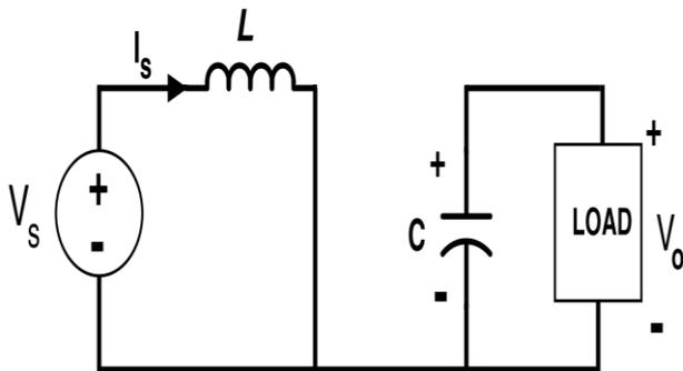
Fig 7: Boost Converter Circuit when Switch S is On (Mode-I)
