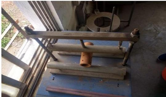
Figure. 5.7 Arrangement of Pipe for Flexural Strength Test
