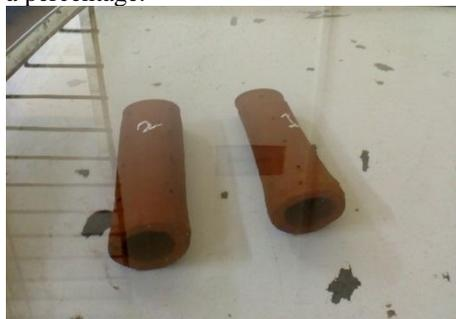
**Figure.5.6 Water Absorption Test**
