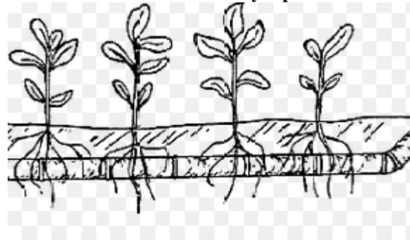
Figure.1.2 Subsurface Porous Clay Pipe Irrigation
