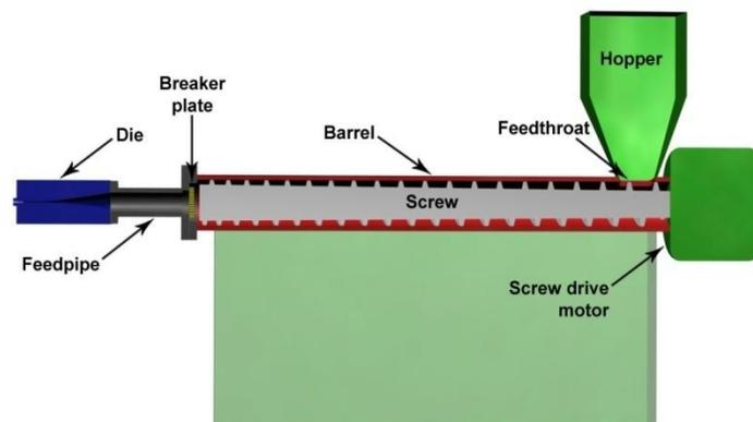
Figure.1. Screw extrusion process
