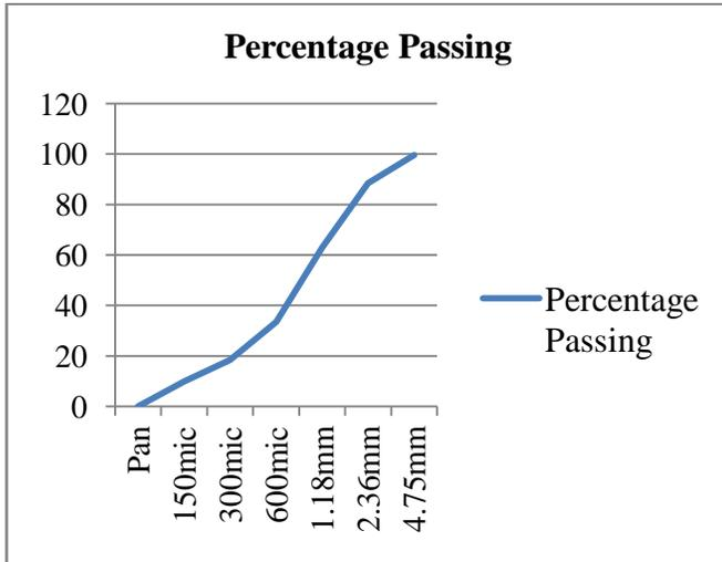
**Figure.1. Sieve Analysis of Fine Aggregate**
