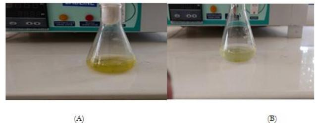
Figure.15. photographs of before and after 9 days of incubation of YELLOW GG dyes.
