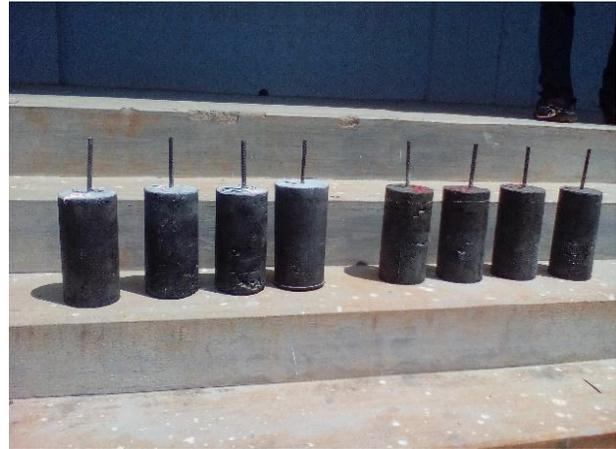
(Impressed current technique experimental setup)
