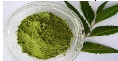
**PONGAM: (Derris indica)** - Flavonoids content in pongam act as corrosion inhibitor. Pongam is taken and the leaves are powdered. Then they are dissolved in the ethanol for dissolving and kept in both higher and lower concentration. Then they are made to evaporate and the thick concentration liquid is taken as the inhibitor.
