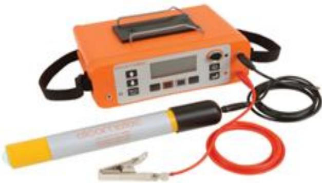
It is an electrochemical method for corrosion rate measurement is the simplest monitoring technique. In this test copper – copper sulphate half cell was used according to ASTM – C 876-87 G3.
