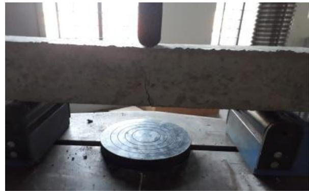
Figure.3. Flexural tests conducted in lab
