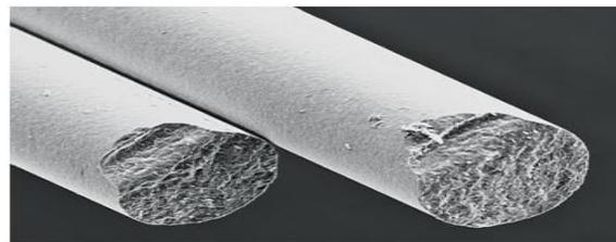
The low density and high specific mechanical properties of aluminum metal matrix composites (MMC) make these alloys one of the most interesting material alternatives for the manufacture of lightweight parts for many types of vehicles. With wear resistance and strength equal to cast iron, 67% lower density and three times the thermal conductivity, aluminum MMC alloys are ideal materials for the manufacture of lightweight automotive and other commercial parts.
