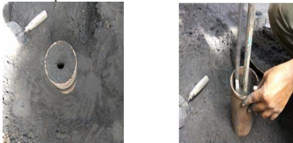
**Fig 3.3 Preparation of Gating System**
