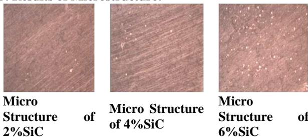
Microscopy of different composites materials such as Al+2wt%SiC, Al+4wt% SiC, Al+6% are shown. One of the most important considerations in the fabrication of metal matrix composites (MMCs) materials is the uniform dispersion or distribution of the reinforcement particles.
