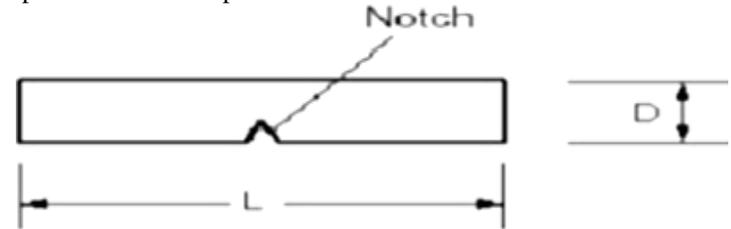
**Fig 3.13 Dimensions of Impact Test Specimen**
