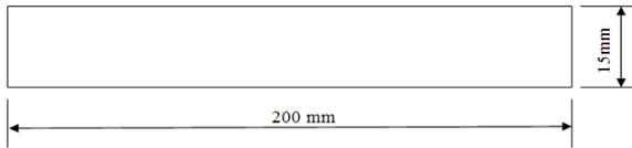
**Fig 3.11 Specifications of Tensile Test Specimen**
