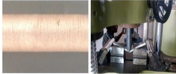
Specimen before and after Flexural Test
