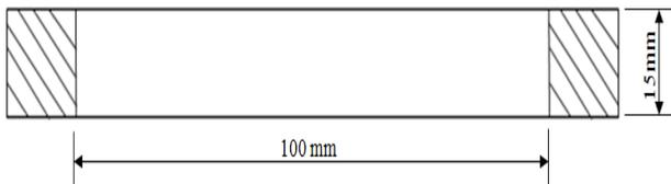
**Fig 3.12 Dimensions of Flexural Test Specimen**
