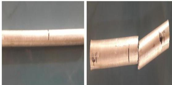
Specimen before and after Tensile Test
