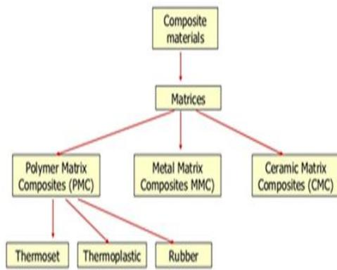
**Fig.1.2 Classification Based on Matrices**
