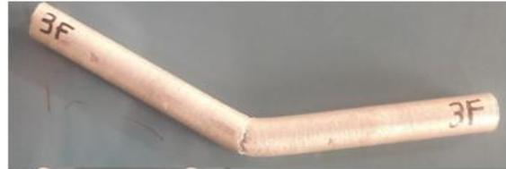
Specimen after Flexural Test
