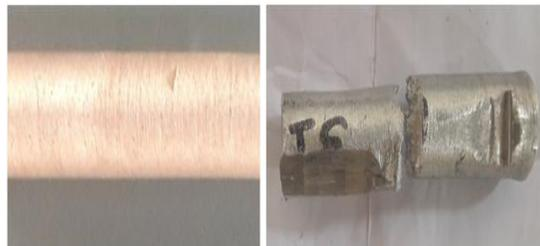
Specimen before Impact Test      Specimen after Impact Test
