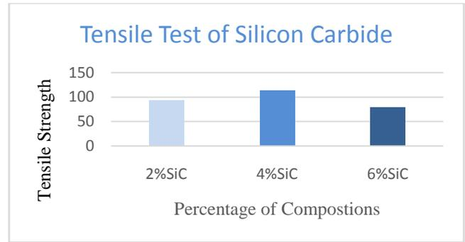
From the graph it can be observed that the tensile strength of the composites are increased to an extent and then decreased. It can be observed that the increase in the filler content contributes in increasing the tensile strength of the
