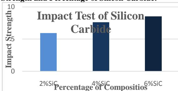
The Izod impact test, also known as the Izod v-notch test, is a standardized high strain-rate test which determines the amount of energy absorbed by a material during fracture. This absorbed energy is a measure of a given material's toughness.
