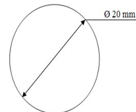
**Fig 3.14 Dimensions of Specimen for Hardness Test**
