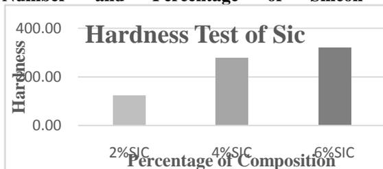
Graph 4.4 shows, the hardness behavior of composites. It can be observed that hardness shows increasing trend with increasing percentage of SiC particulates. This hardness increase was observed from 121 BHN for sample 1 to 319 BHN at 6 wt% SiC reinforced composite (A3) at room condition. This could be due to the presence of SiC particulates which are hard in nature.
