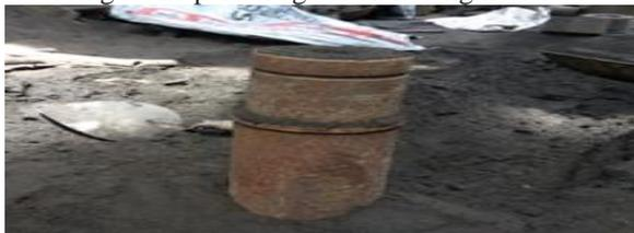
**Fig. 3.4 Incorporate the Pattern and Sand in a Gating System**
