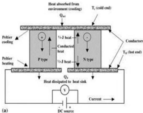
**Figure.5. Schematic diagram of thermoelectric cooling**
