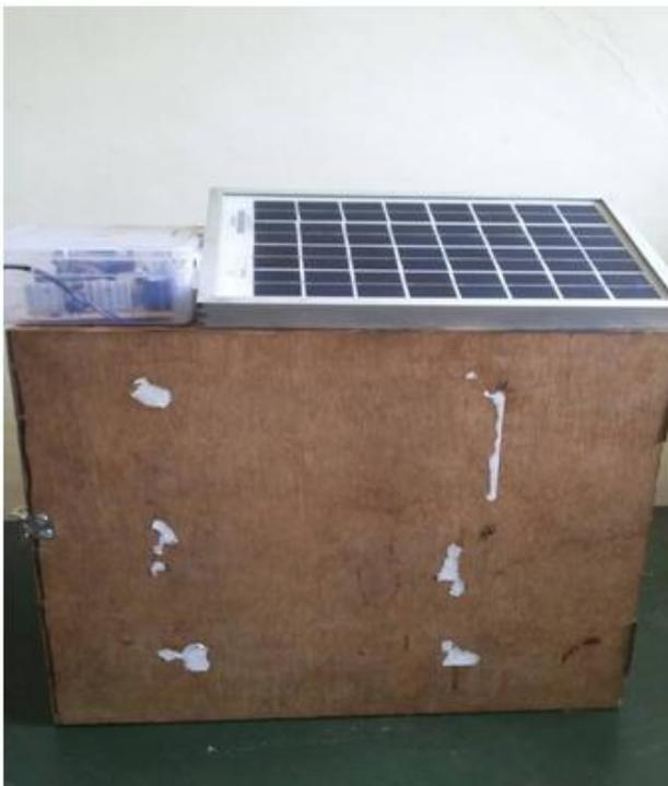
**Figure.1.Fabricated Thermo- Electric Refrigerator system powered by solar energy**
