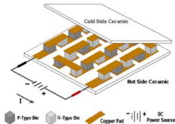
**Figure.2. Internal construction of thermo- electric module (Adapted from ADVANCED THERMOELECTRIC · One Tara Boulevard · Nashua, NH 03062 · USA)**
