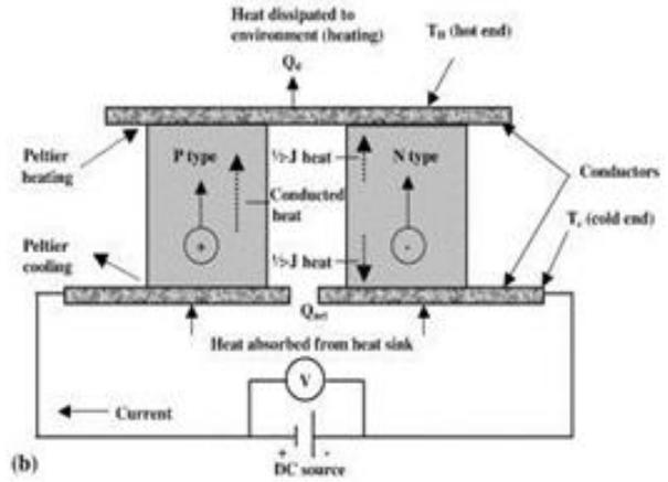
**Figure.6. Schematic diagram of thermoelectric heating**
