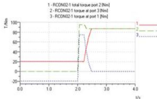
**Changes on Lifting Brake, Load and Motor Torque under the Condition that System Ascends after Stopping**
