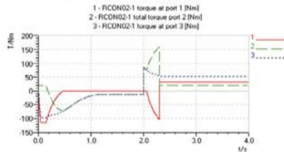
**Changes on Brake,Load and Motor Torque under the Conditon that System Stops during Descension**
