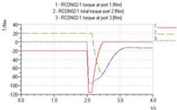
**Changes on Brake, Load and Motor Torque under the Condition that System Descends after Stopping**
