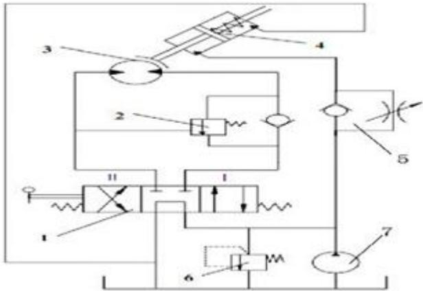
1-Change Valve 2-Balanced Valve 3-Hydraulic Motor 4- Brake Hydro-Cylinder 5-One-Way Throttle Valve 6-Pressure-Control Valve 7- Hydraulic Pump
