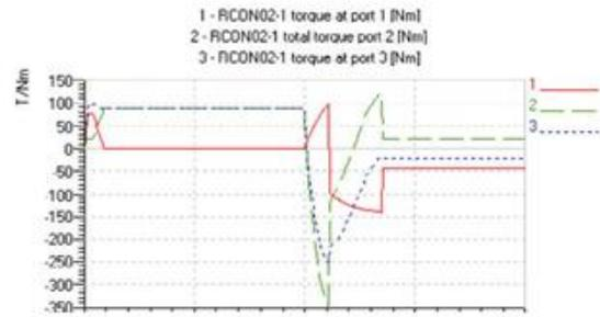
**Changes on Suspend Brake, Load and Motor Torque under the Condition that System Stops during Ascension**
