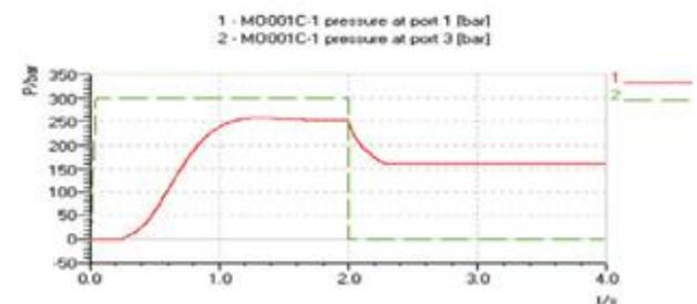
**Pressure Changes of Port1 and Port3 in the Motor**
