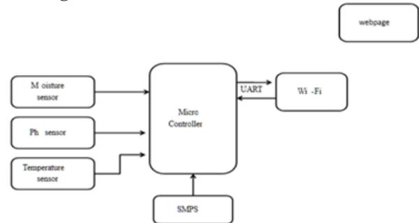
**Figure.1. Block Diagram for proposed model**
