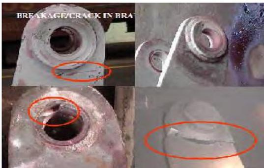
Figure.3. Various Type of Hanger Failure
