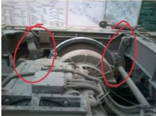
Figure.2. Brake Hanger Assembly
