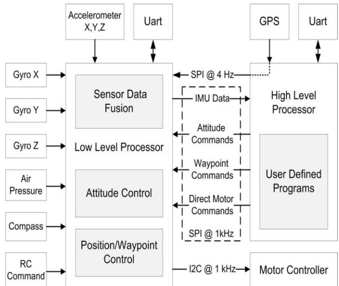
Fig. 2. Electronic architecture: All sensors, except the GPS, are connected to the LLP which communicates via I2C with the motor controllers and via SPI with the HLP.
