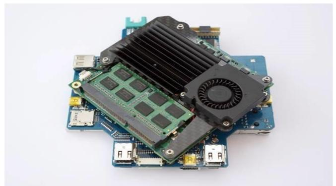
Fig. 3. On-board computer AscTec Mastermind featuring a Core 2 Duo CPU
