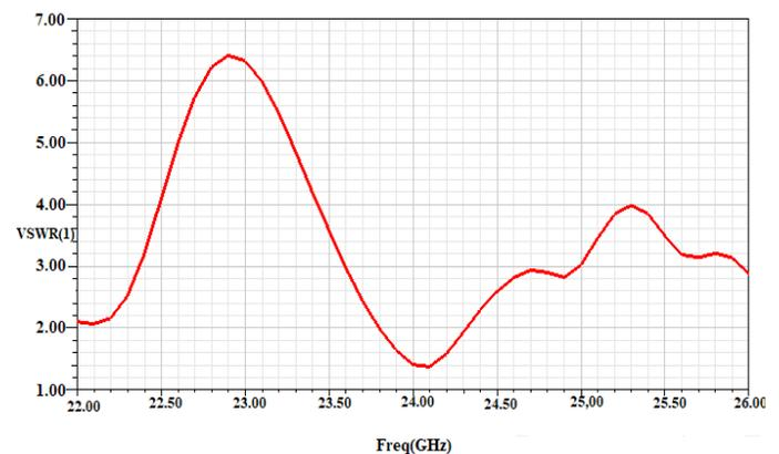
**Figure.4. VSWR of T-shaped Slot antenna**
