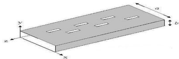
Figure.1. Structure of Slot antenna
