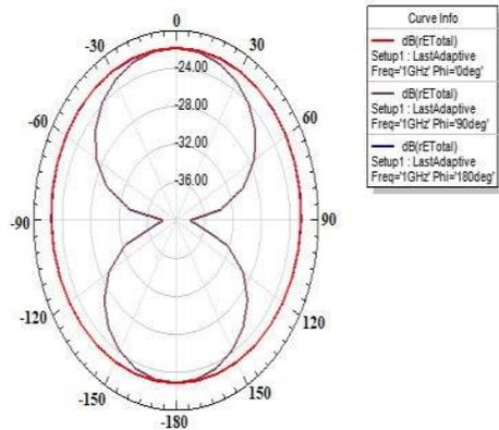
Figure.5. Radiation Pattern of Slot Antenna
