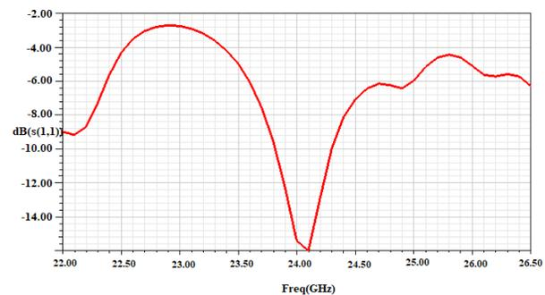
**Figure. 3 Return loss of T-shaped Slot antenna.**
