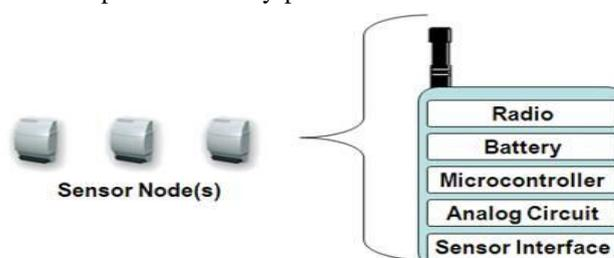
**Figure.2. Components of a WSN Node**
