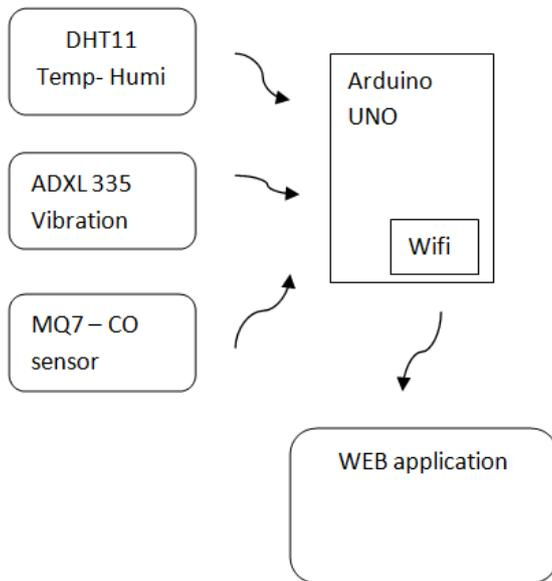
**Figure .3. Block Diagram WSN system**
