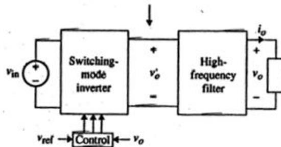
Figure.3. Single phase inverter with filter
