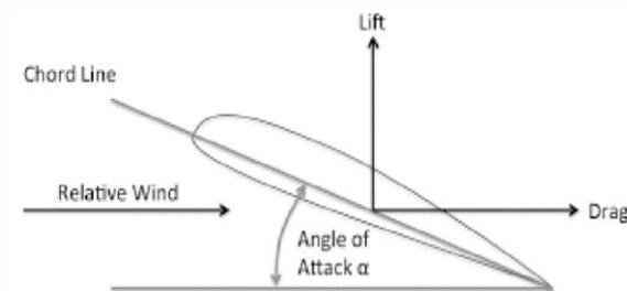
Figure.1 Lift and Drag force
