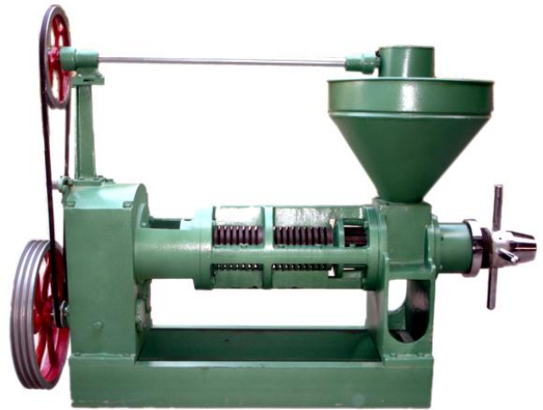
Figure 2.1 Manila Tamarind and Custard Apple oil Seed crushing machine
