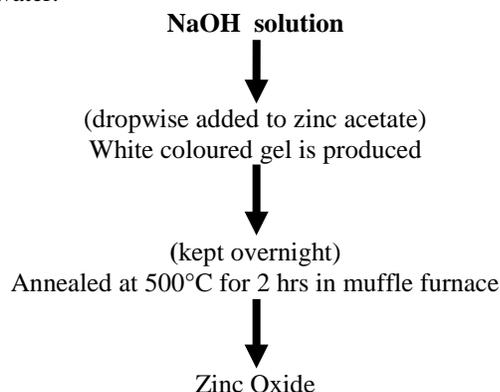
Figure.2. Flow chart for the preparation of ZnO
