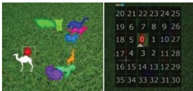
Figure.5. A Click Animal Image(Left) and 6*6 Grid (Right) Determine by Red Turkey's Bounding Rectangle
